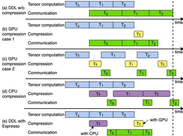
**Figure 2.** A DDL example with different compression strategies. (a) is the baseline; (b) reduces the iteration time, but it is not optimal; (c) and (d) harm the performance; (e) is our solution and achieves optimal performance. The communication and compression overheads depend on the interactions among tensors. The decompression operations are omitted.
