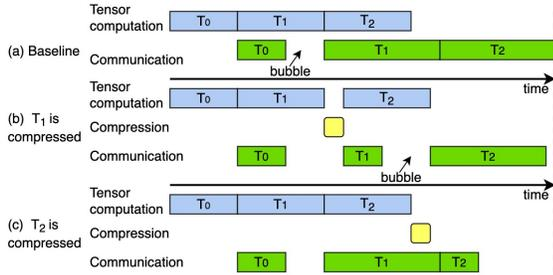
**Figure 9.** (a) shows that tensors communicated before bubbles need no compression.  $T_1$  and  $T_2$  have the same size. In (b),  $T_1$  is compressed and a new bubble is formed. In (c),  $T_2$  is compressed and it reduces more iteration time than compressing  $T_1$ .
