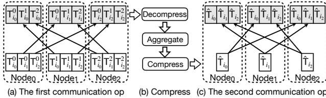
**Figure 4.** A divisible scheme. In (a),  $T_i^j$  is partitioned into 3 parts, i.e.,  $T_{i_0}^j$ ,  $T_{i_1}^j$ , and  $T_{i_2}^j$ . The first communication operation (op) is a shuffle. After Node  $j$  receives the  $j$ th part from other nodes, it decompresses and aggregates them. It then compresses the aggregated tensor and obtains  $\hat{T}_i^j$  for the second communication op.
