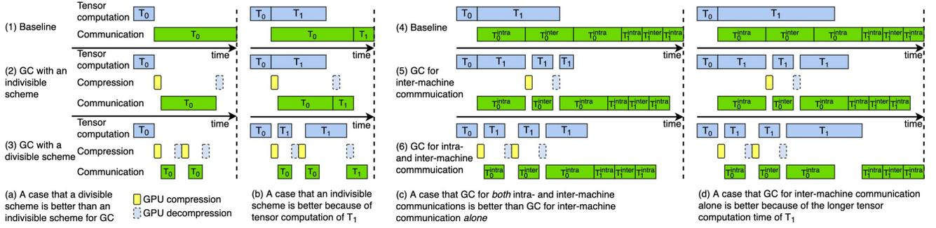
**Figure 5.** (a) and (b) show that the choice of communication schemes depends on the interactions among tensors. Only  $T_0$  is compressed. (c) and (d) show that the decision to apply GC to inter-machine communication alone or to both intra- and inter-machine communications also depends on the interactions among tensors.  $T_i^{intra}$  and  $T_i^{inter}$  are  $T_i$ 's intra- and inter-machine communications.
