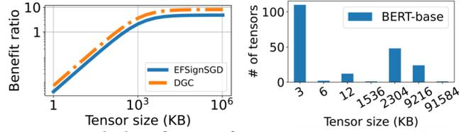
**Figure 10.** The benefit ratio of GPU compression. **Figure 11.** Number of tensors with the same sizes.
